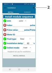
During activation, 3 parameters are requested: the serial number of the mechanical meter, the pulse weight and the reading of the volume measured by the meter expressed in litres.
