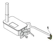
Fasten Arrow<sup>WAN</sup> to a pipe (2) using the clip (3) supplied as an accessory. When installing the device on buried manholes, secure it as close as possible to the surface.
