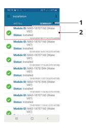
Clicking an item from the list of installed modules (2) allows for viewing the details (3) relative to the installation.
