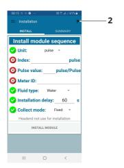
During activation, 3 parameters are requested: the serial number of the mechanical meter, the pulse weight and the reading of the volume measured by the meter expressed in litres. Once these preliminary operations have been completed, proceed as follows:
